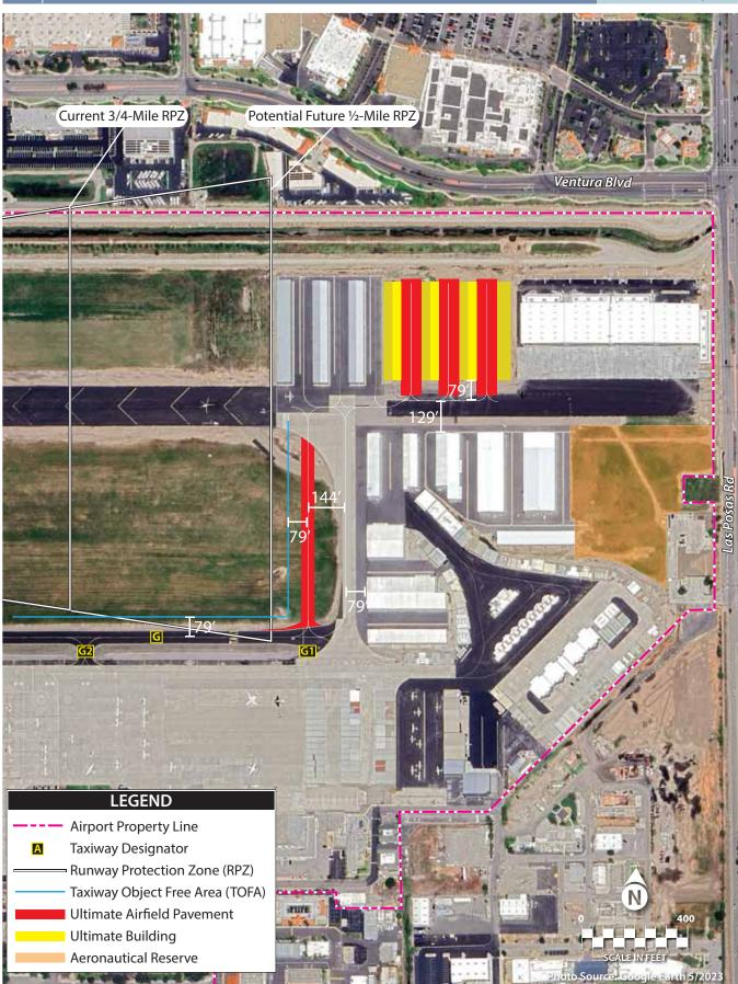
Larger conventional and medium sized box hangars intended to accommodate the turbine aircraft are expected to be proposed within areas identified as aeronautical development/redevelopment or aeronautical reserve. These areas are also expected to accommodate hangars to house aircraft expected beyond the forecast period of this ALP Update. Detailed concepts for development beyond this forecast horizon will be the subject of a future study.
